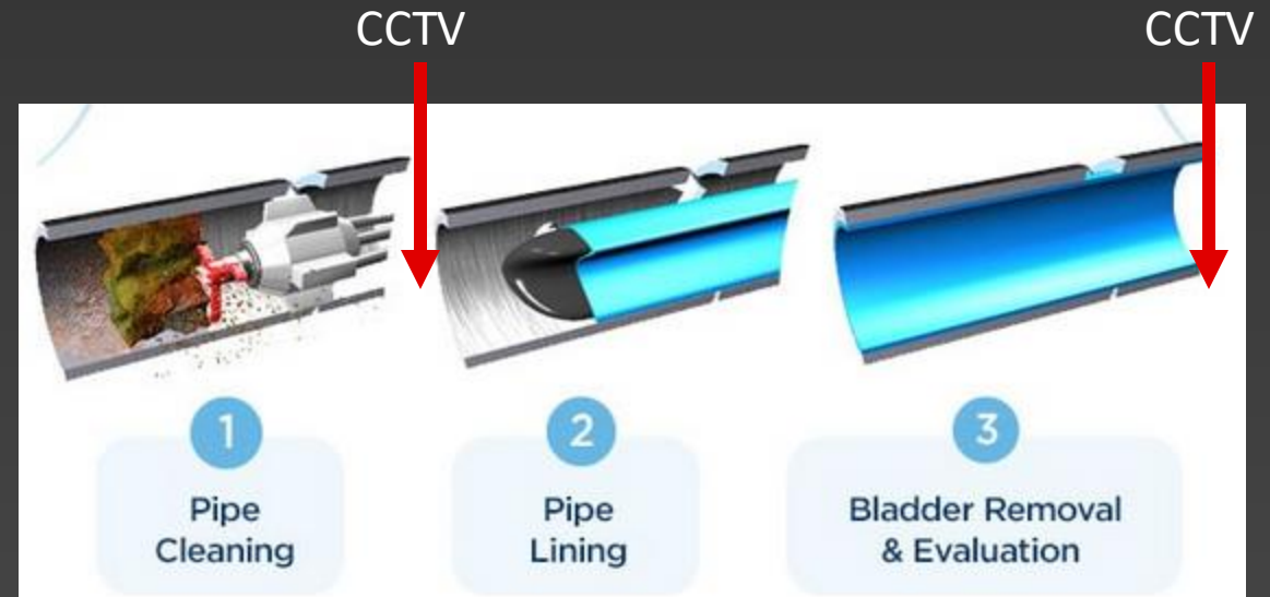
General Work Process (Courtesy of Nu-Flow)
